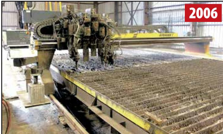
ESAB AVGXP2-VIS PC CNC PLASMA AND FLAME CUTTING TABLE
